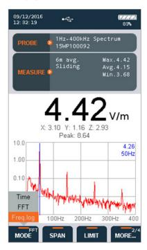
Select the "Freq. log" mode directly on the "MODE" menu, then specify the desired frequency:
