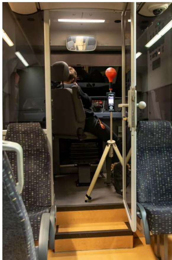
Figure 2: SMP2 + WP400 mounted on a tripod at a height of 1.5 m in the train driver cabin near the driver's seat.
