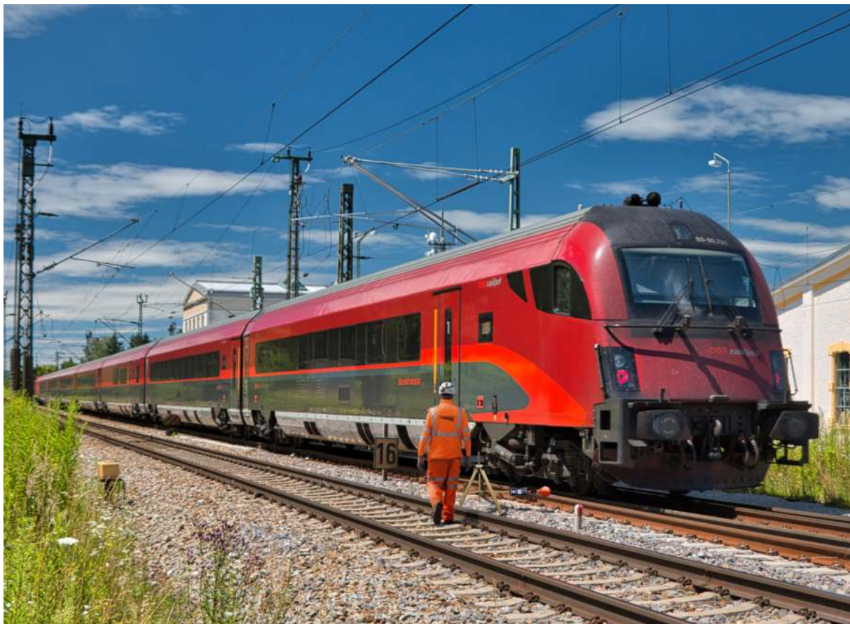
Figure 4: Assessment of the exterior of the rolling stock with the SMP2 mounted on a tripod at 50 cm in the area closest to the emission source.
