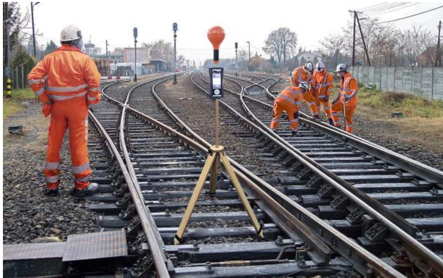
Figure 5: SMP2 mounted at 1.5 m on the center of the train track.
