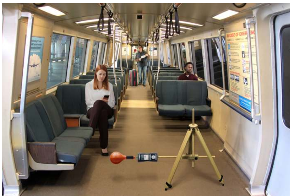
Figure 3: SMP2 mounted on a tripod at 1.5 m ( top image ) and at 30 cm distance from where the public may be for assessment in public areas. Using the horizontal extension, the SMP2 can also be placed on the tripod disk at a height of 0.3 m ( bottom image ).
