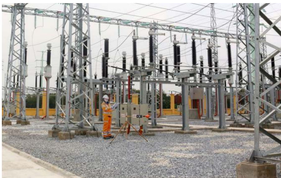
Figure 6: The SMP2 mounted in a railway electric traction substation at a height of 0.9 m.
