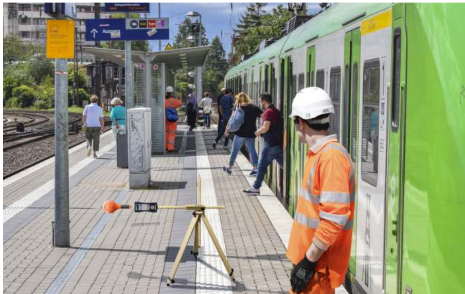
Figure 7: Assessment of the train station platform with the SMP2 mounted at recommended heights using the horizontal tripod extension.
